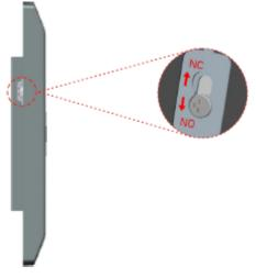
Alternate fail safe and fail secure(adjustable) Procedure:
